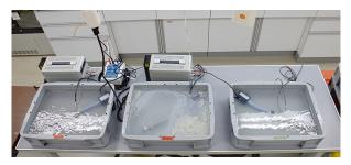
Fig. 5. Electro-degradation of nutrient solution after a without plant experiment for 24 hours. Alternating current—electrodegradation (AC-ED) was applied at a 50% duty ratio, 2.0 amperes alternate current, and 14.0 volts (left). Direct current electro degradation (DC-ED) was applied at 2.0 amperes and 18.0 volts (middle). Control-without ED application; the nutrient solution was flowed using the pump only (right) (Talukder et al., 2019).
